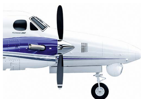
Side view of the utility nose with a camera lift kit
