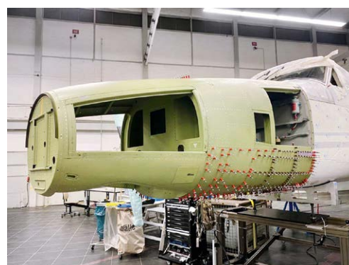
Utility nose with lift kit during installation
