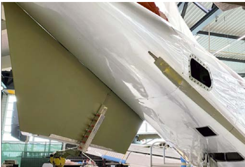
Aft mission strakes installation in progress
