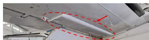
Under-wing wiring duct for wire routing from hardpoint to fuselage
